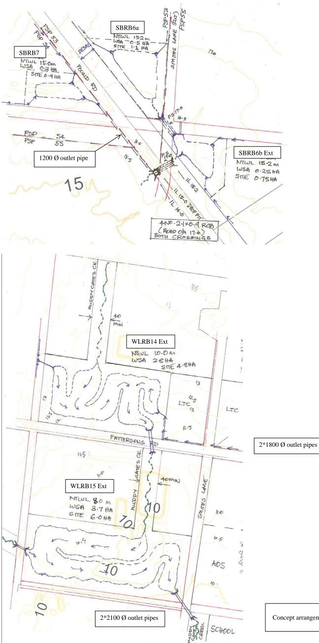
Figure 7 (Sheet 1 of 2) Concept arrangements for proposed stormwater management assets in Muddy Gates Creek catchment
