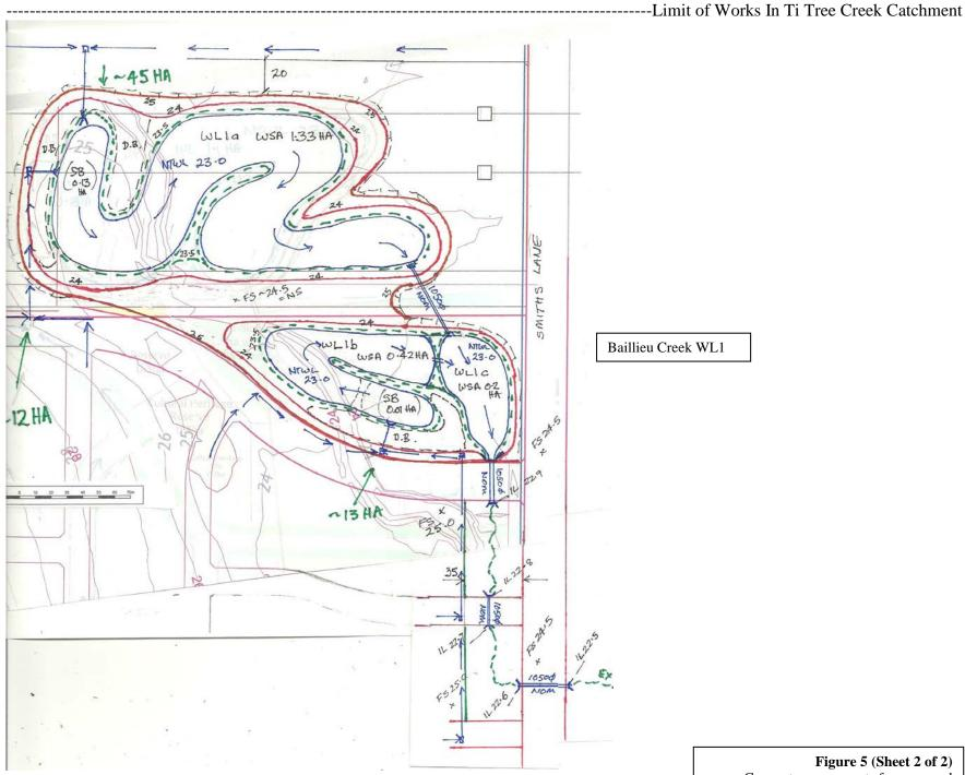
Figure 5 (Sheet 2 of 2) Concept arrangements for proposed stormwater management assets in Ti Tree Creek and Baillieu Creek catchments (moving west-east sequentially)
