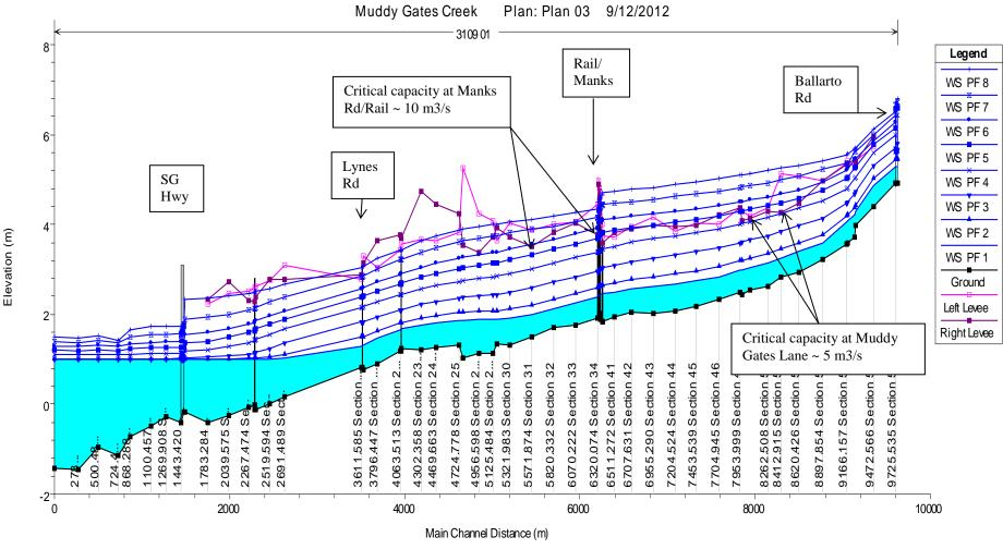
Profiles for 20, 15, 10, 7.5, 5, 2.5, 1 and 0.5 m3/s respectively, for threshold capacity checks (Note: profiles above confining levees are hypothetical)
